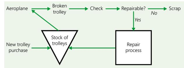
Figure 1. Trolley process
